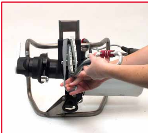
3. Remove the strop from upper anchorage point.
