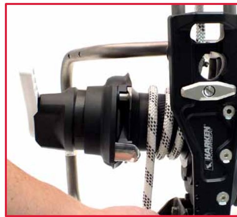
8. Wind the rope clockwise around the winch drum.
