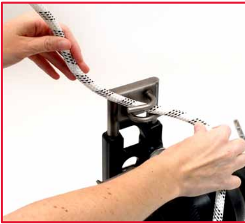
5. Pass the primary rope inside the pins.
