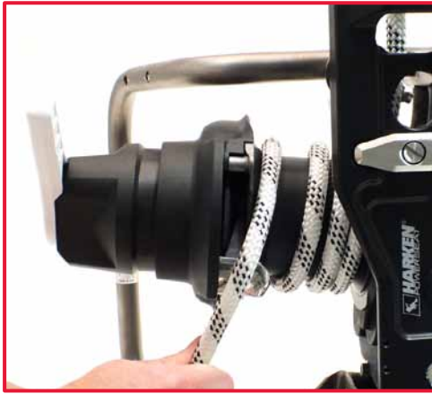
9. Pass the rope over the stripper arm.
