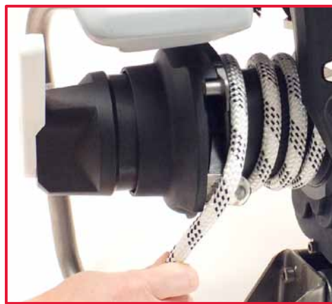
8. Pass the rope over the stripper arm.
