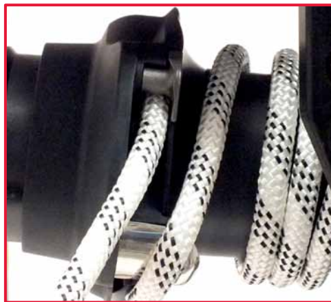
10. Position the rope inside the stopper.
