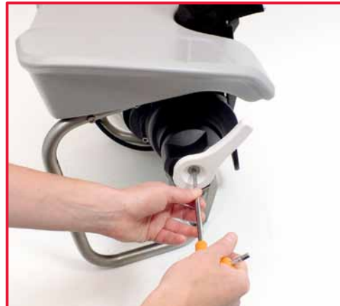
3. Tighten the control lever screw.
